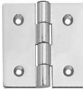
#42.578 - 75 mm x 75 mm x 2.5 mm; medium duty, for cabin doors 316 stainless steel. For screws 4.5/5 mm
